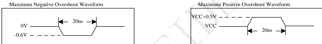
Figure 5-1 Maximum Overshoot Waveform
